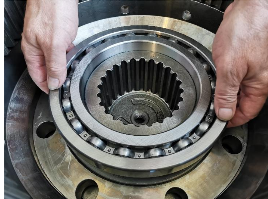
Assembly of new bearings and seals
