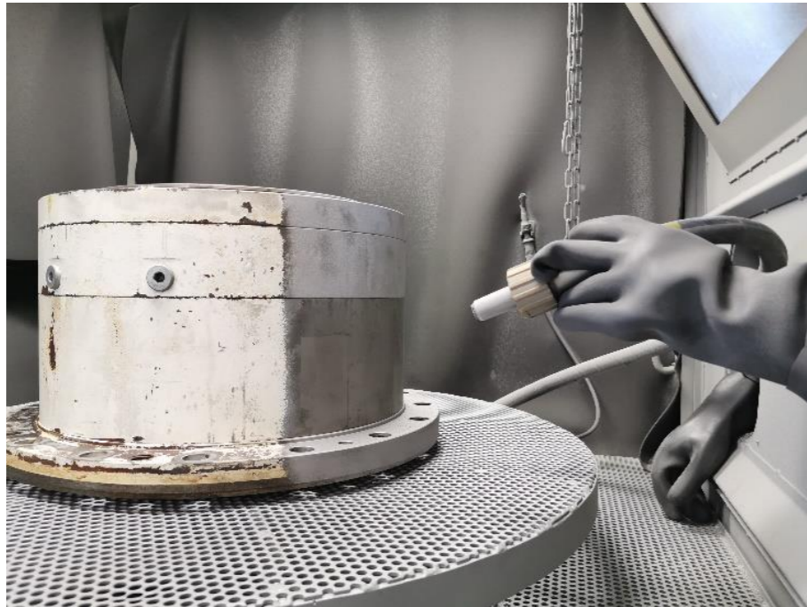
Conservative sand blasting for removal of painting
