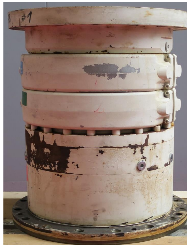
Gearbox before refurbishment
