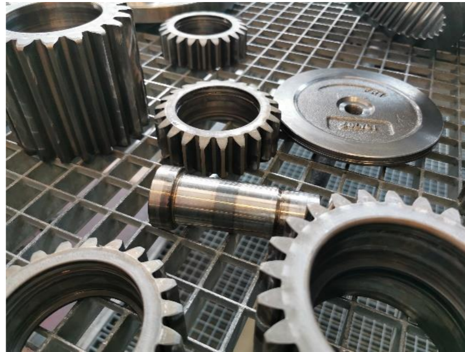
Washing of the components in specific cleaning station
