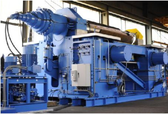
Planetary gearboxes as top- and bottom roll drive on a steel bending machine
