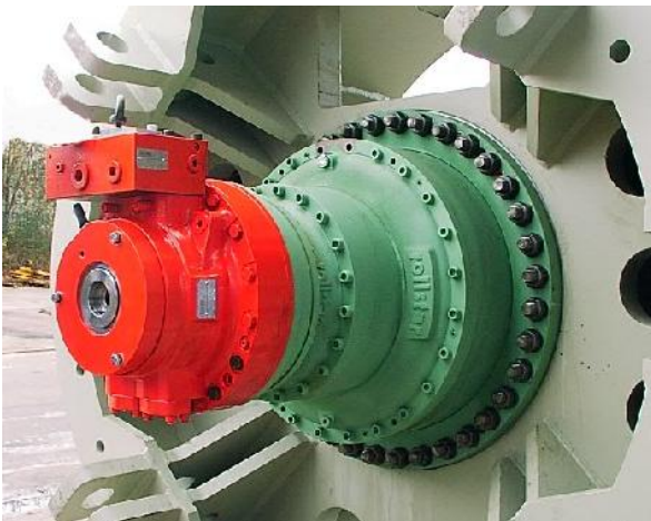
Planetary gearbox as a central cutter wheel drive on a tunnel boring machine
