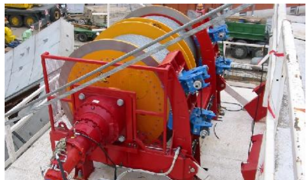
Planetary gearbox as a winch drive for shaft systems in the mining industry
