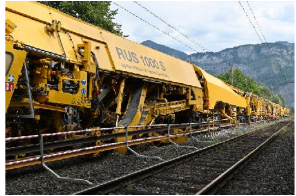
Hydraulic motors as traction- and conveyor belt drive on a track construction machine Source: Plasser & Theurer
