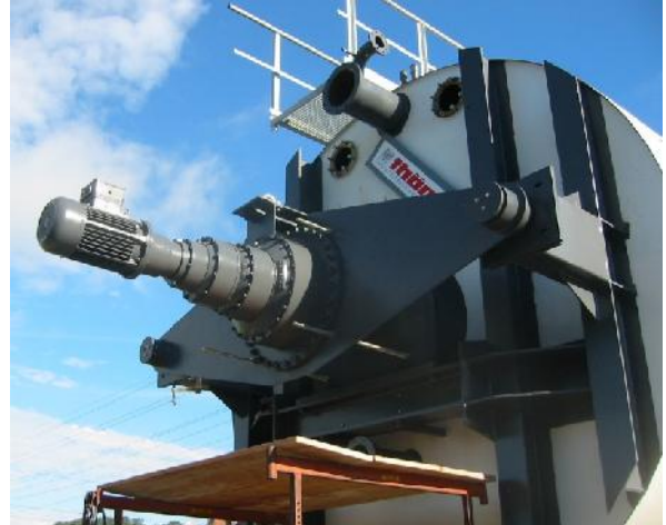
Planetary gearbox with electric motor as an agitator drive in the fermentation plant industry
