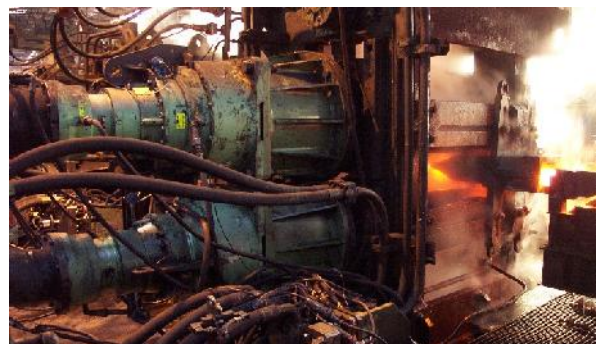
Planetary gearbox as rolling mill drive in the iron and steel industry
