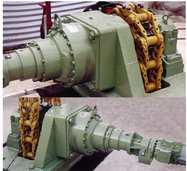
Planetary gearboxes with electric motor as a top and bottom drive of a chain drive
