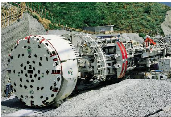
Planetary gearboxes as cutter wheel drives on a tunnel boring machine
