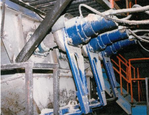
Planetary gearboxes in the paper industry as mill drives
