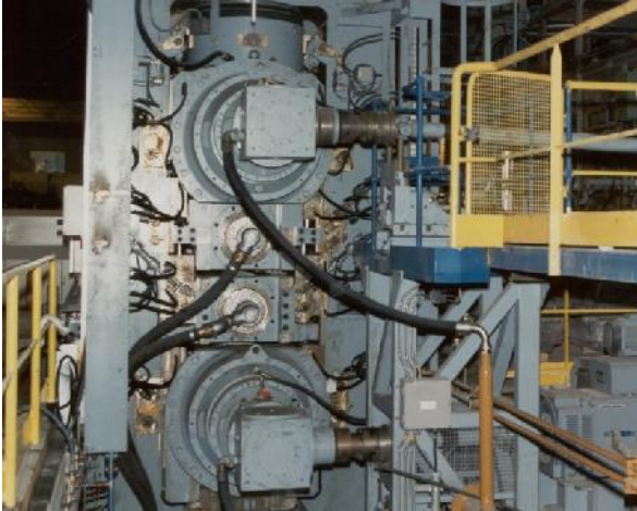
Planetary gearboxes in the aluminium industry, here with additional angular gearbox
